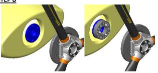
Install the stacked whole on the propeller-shaft (or on the corresponding adaptor spacer corresponding). **Tighten moderately.**
