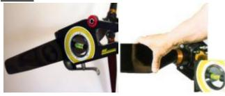
Adjust the pitch angle of the blades with the adjusting tool. See the item **4.4. Adjusting the blade angle of the propeller**.
