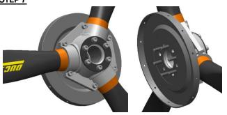
From the back, position the spinner mounting plate according the screws. Be careful to respect the direction of the plate. <u>Step 8</u>
